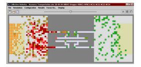
Figure 4: Positioning of all the virtual markers (dark squares) for the goal *reach laying zone* in a difficult environment (with deadends).
